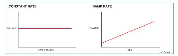
Pump Operation Profiles available on the KDS Legato 110, 111 or 180 pump.
