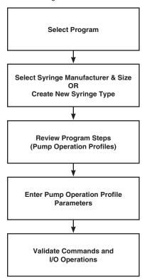
The software provides the user with a variety of prompts and warnings to help guide the setup of programs. For example, if a pump Program incorporates steps that exceed the capacity of the defined syringe, the system will prompt you that parameters are out-of-range. The system also prompts users if required values are not entered.
