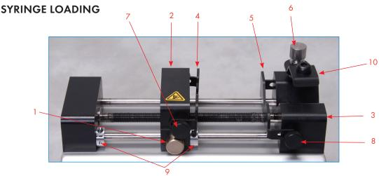
The Legato 100 Series can accommodate up to two syringes. Depending on the mechanism, any type of syringe, glass, plastic or stainless steel can be used. The pump can accommodate from 0.5  $\mu$ l to 60 ml single syringe and 0.5  $\mu$ l to 10 ml dual syringe. The syringe barrel clamp should be flipped for syringes smaller than 30 ml. For syringes larger than 30 ml, the syringe clamp should be used as shown.
