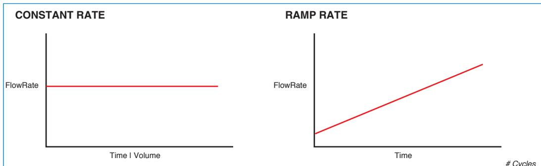
Pump Operation Profiles available on the KDS Legato 110, 111 or 180 pump.
