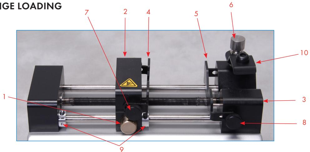
The Legato 100 Series can accommodate up to two syringes. Depending on the mechanism, any type of syringe, glass, plastic or stainless steel can be used. The pump can accommodate from 0.5 µl to 60 ml single syringe and 0.5 µl to 10 ml dual syringe. The syringe barrel clamp should be flipped for syringes smaller than 30 ml. For syringes larger than 30 ml, the syringe clamp should be used as shown.
