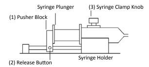
To facilitate loading, the pusher block (1) can be released from the leadscrew and manually moved along the guide rods to accommodate the syringe.
