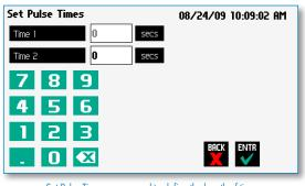
Set Pulse Times screen used to define the length of time the pump will operate at each pulse step level
