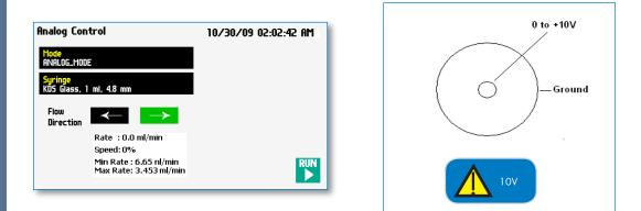
Turning the Potentiometer CW will increase the motor speed (center pin is 10 VDC) and turning the Potentiometer CCW will decrease the motor speed (center pin is 0 VDC).
