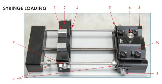
The Standard Legato 200 Series can accommodate up to two syringes. Any type of syringe, glass, plastic or stainless steel can be used. The pump can accommodate from 0.5 ul to 140 ml syringes. The syringe barrel clamp should be flipped for syringes larger than 30 ml. For syringes smaller than 30 ml, the syringe clamp should be used as shown.
