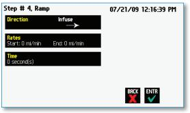
Step Definition screen for a Ramp Rate profile
