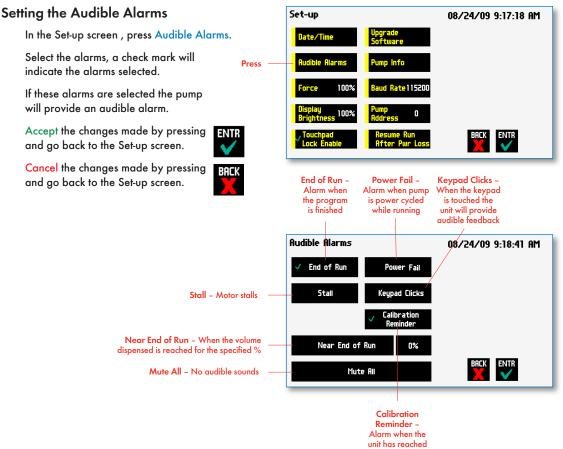
Alarm when the nit has reached its calibration due date
