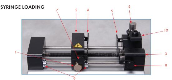
The Legato 950 OEM Series can accommodate up to two syringes. Depending on the mechanism, any type of syringe, glass, plastic or stainless steel can be used. The pump can accommodate from 0.5  $\mu$ l to 60 ml single syringe and 0.5  $\mu$ l to 10 ml dual syringe. The syringe barrel clamp should be flipped for syringes smaller than 30 ml. For syringes larger than 30 ml, the syringe clamp should be used as shown.
