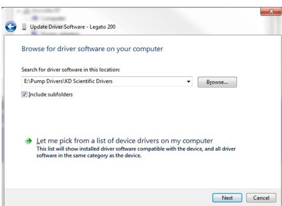
4. Click Browse and navigate to the pump drivers folder located on the CD supplied with the pump. Select the file KDS Scientific USB-CDC.inf. Make sure the Include Subfolders box is checked and then click Next.
