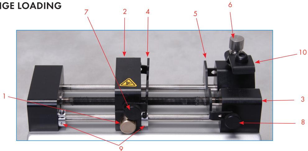
The Legato 950 OEM Series can accommodate up to two syringes. Depending on the mechanism, any type of syringe, glass, plastic or stainless steel can be used. The pump can accommodate from 0.5  $\mu$ l to 60 ml single syringe and 0.5  $\mu$ l to 10 ml dual syringe. The syringe barrel clamp should be flipped for syringes smaller than 30 ml. For syringes larger than 30 ml, the syringe clamp should be used as shown.
